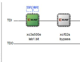
Right click on the `xc3s500e` chip and select *Assign new configuration file* and choose the `lab1.bit` file. Then right click again, and choose *Program* to download the bitstream file to the FPGA. If everything works right, you should see the numbers on your seven-segment LCD display.
